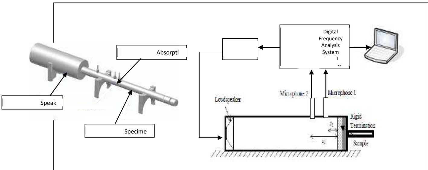
Figure 1: Schematics of an impedance tube used for measurement of acoustic absorption coefficient
