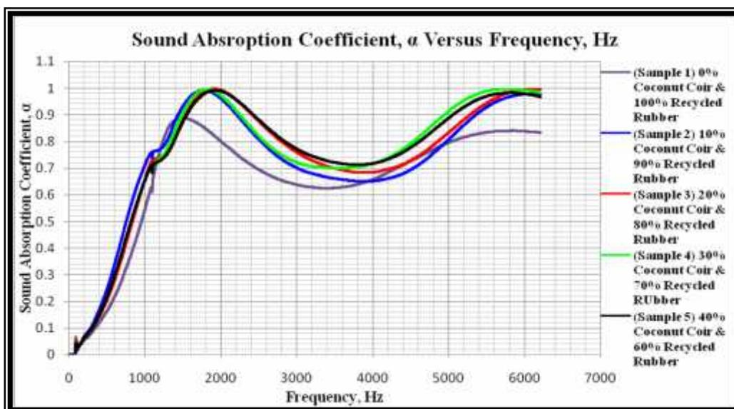
Figure 2: Sound absorption coefficient for various compositions with 25 percents of natural latex
