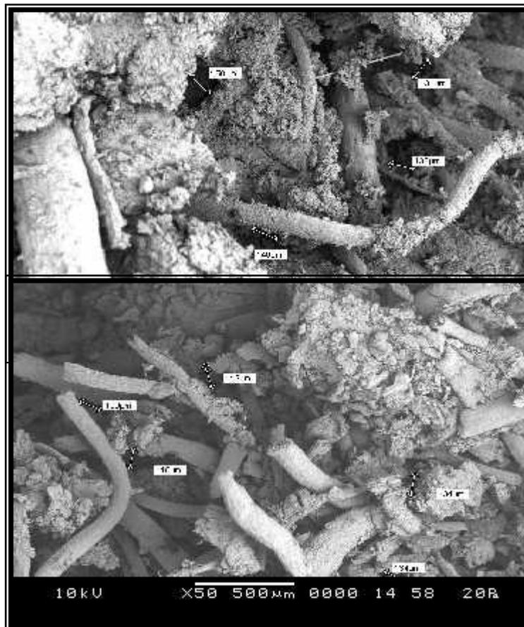
Figure 8: Microstructure view for panel board with 35 percent of natural latex
