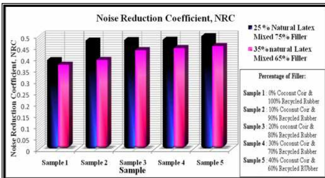
Figure 4: Noise reduction coefficient for various compositions of filler and resin
