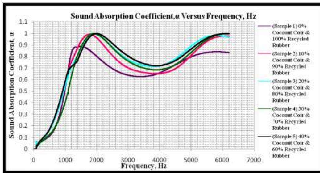
Figure 3: Sound absorption coefficient for various compositions with 35 percents of natural latex
